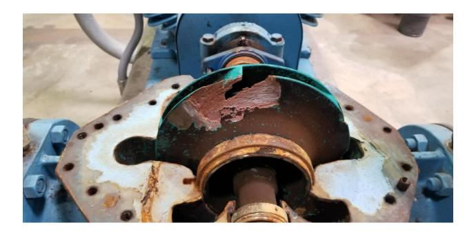
Once the pump casing was opened up it was found that the impeller had degraded and pieces of the impeller had worn out and broken off. Bodine of Decatur will be to the plant to pick up the pump and install a new impeller.
