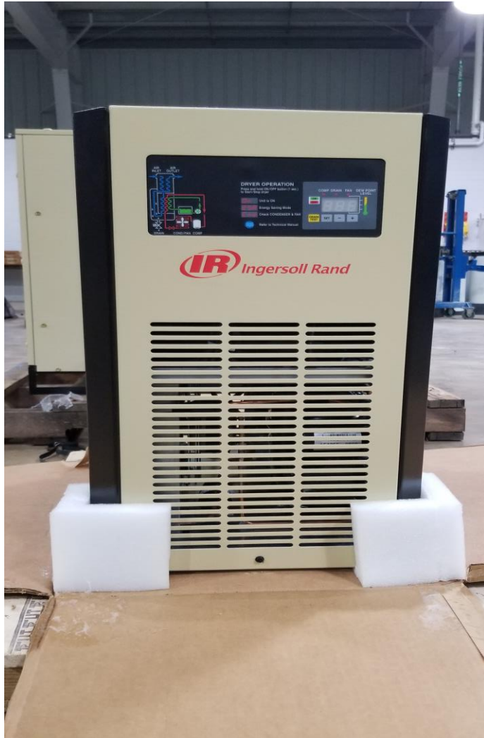
The new air drier for the air control system
